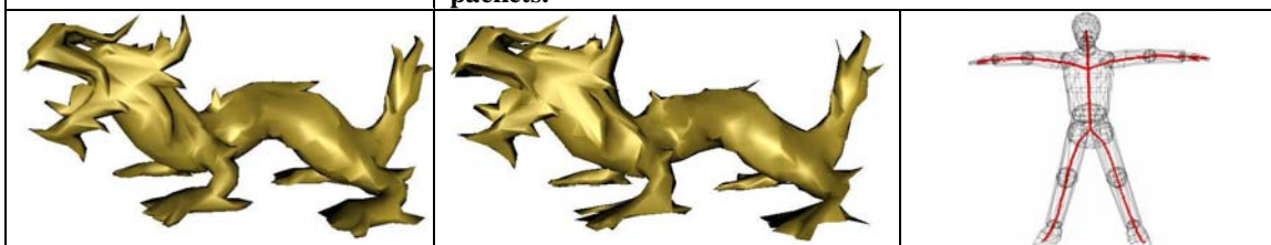
Figure 13: Visual quality is satisfactorily preserved by the curvature-driven probabilistic transmission strategy: (left) original 3D model and (right) reconstructed model using a network packet loss rate of 55%.
