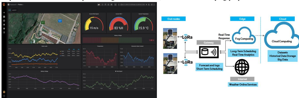
Figure 4 On the left, a dashboard to visualize the data collected by our device. On the right, a three-layered cloud architecture for IoT energy-neutral devices.
